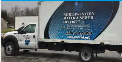
The District continues to use technology to work smarter. Our new sewer inspection truck allows us to see the condition of our sewer and lateral lines without excavation. The truck is equipped with two cameras that can record and feed video footage of what lies within the lines. "Prior to acquiring the truck, The District would have to hire a company to *(continued next page)*
